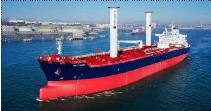
Rendering of the retrofitted rotors aboard the MR tanker (Norsepower)
